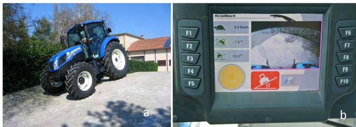
Figure 2. Tractor on the inclined plane during the static test (a); display of the system visualizing the alarm signal (b)
