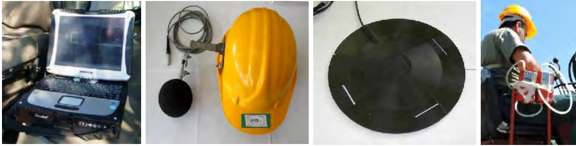
Figure 3. From left to right: “Soundbook” system for noise; microphone mounted on the operator’s safety helmet; seat pad accelerometer; air personal samplers.
