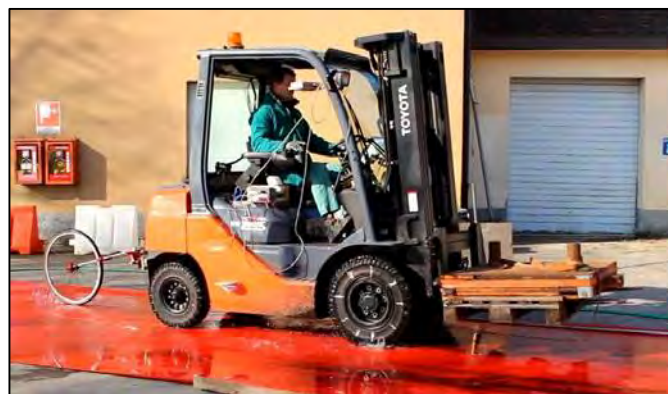
Figure 3. Example of the equipment layout of the test on PVC.
