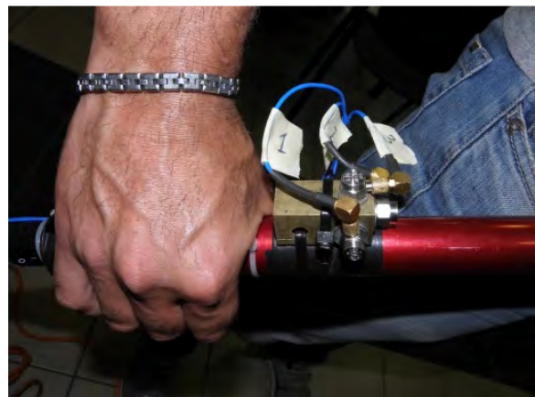
Figure 2. Accelerometer positioning on the bar and reference axes (1: x-axis; 2: y-axis; 3: z-axis).
