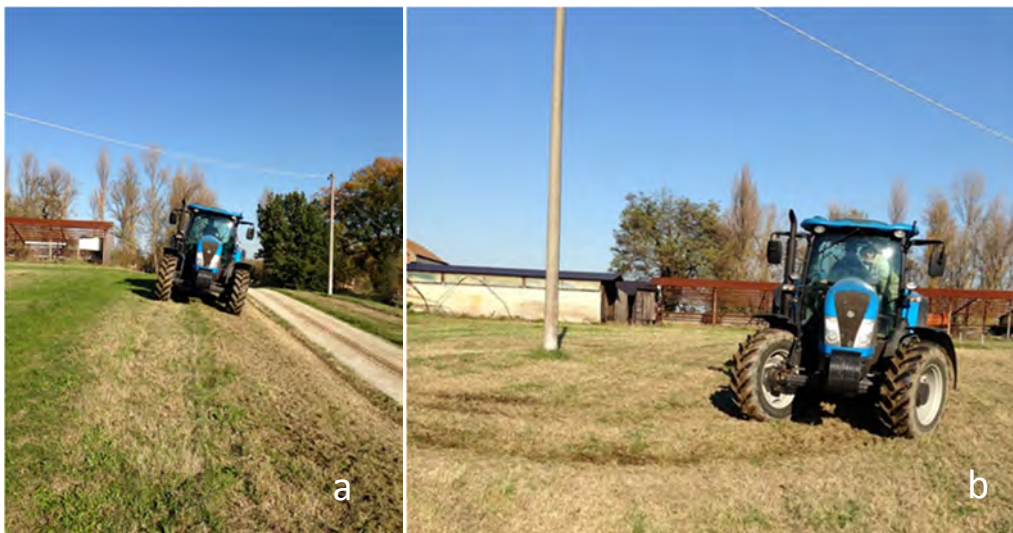
Figure 3. Test in field to evaluate the roll angle (a) and the steering condition (b)
