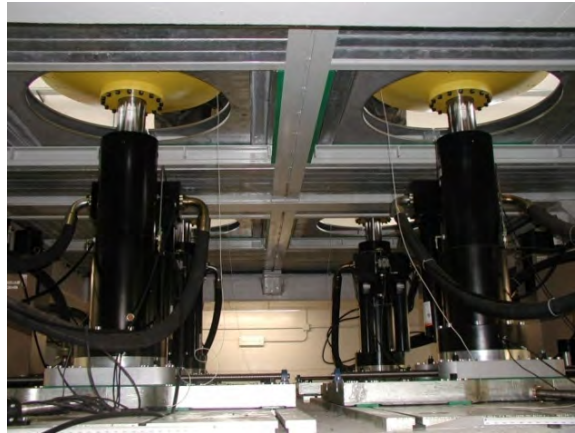
Figure 1. One actuator of the four poster was used for validating the application INTRAC-safety.
