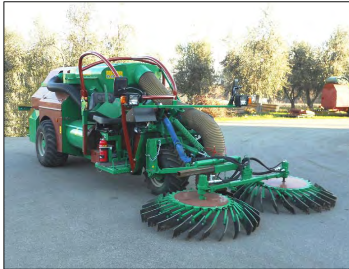
Figure 4. The harvesting vacuum machine mod. Facma 300 S, equipped with 2 rotating sweeps
