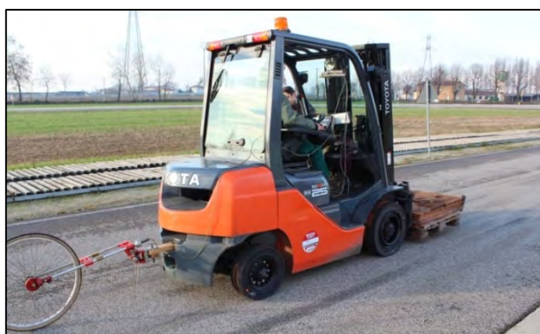
Figure 1. The forklift truck during one of the tests carried out on asphalt with the T_95 set of tires.
